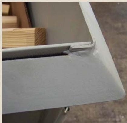
**Welded reinforcing angle all along the top edge**
