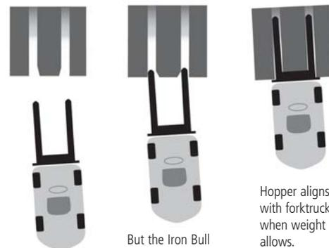
Here forklift is misaligned with hopper.
