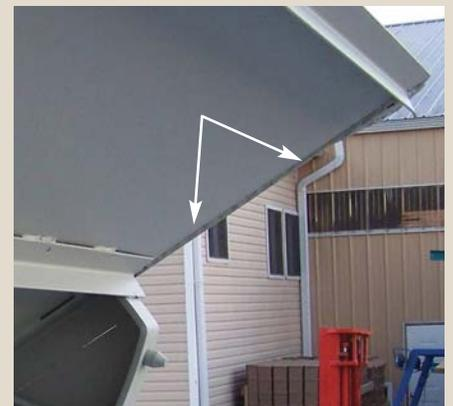
**Sides of hopper extend down past hopper bottom for added strength**
